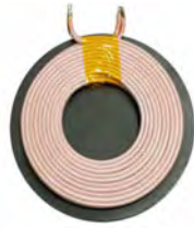
A5 Transmitter coil 2 layers, Alpha winding ID: 20.5 OD: 43 Wire: 0.08*105P Inductance: 6.3+/-10%uH
