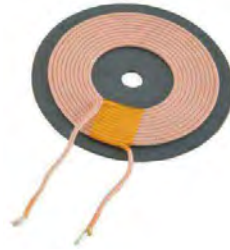
A11 Transmitter coil 1 layer, common winding ID: 20.5 OD: 43 Wire: 0.08*105P Inductance: 6.3+/-10%uH
