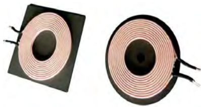
A10 Transmitter coil 2 layers, Alpha winding ID: 20.5 OD: 43 Wire: 0.08*105P Inductance: 24+/-10%uH
