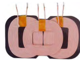
A6 Transmitter coil 1 layer, common winding ID: 20 OD: 42.5 Wire: 0.08*105P Inductance: 7+/-10%uH
